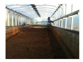
The Earth Flow has an integrated mixing system that allows the compost to be mixed on a daily basis (2-4 times per day). The Traveling Auger is the true magic of the Earth Flow and really is the optimum technology for hot food waste composting. The traveling auger provides seven different functions that facilitate the hot composting process:
